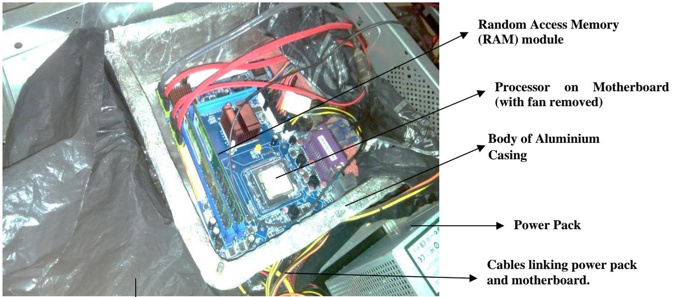
Plastic Casing realized via flexible plastic wrapping.
