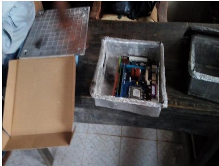
**Figure 3 – Motherboard being placed in Aluminium casing.**
