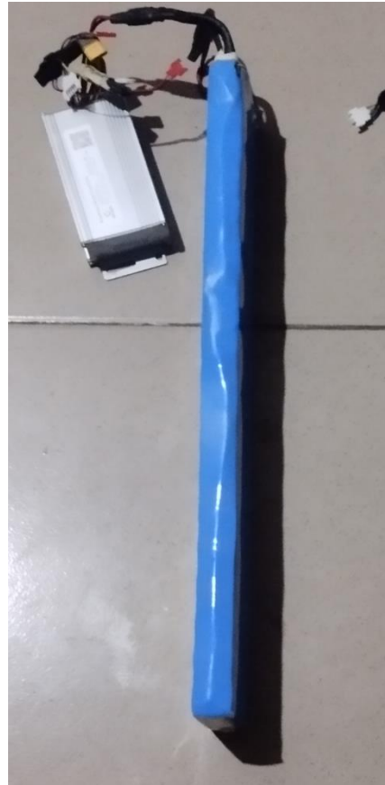
Figure 2: Speed controller and Lithium iron battery
