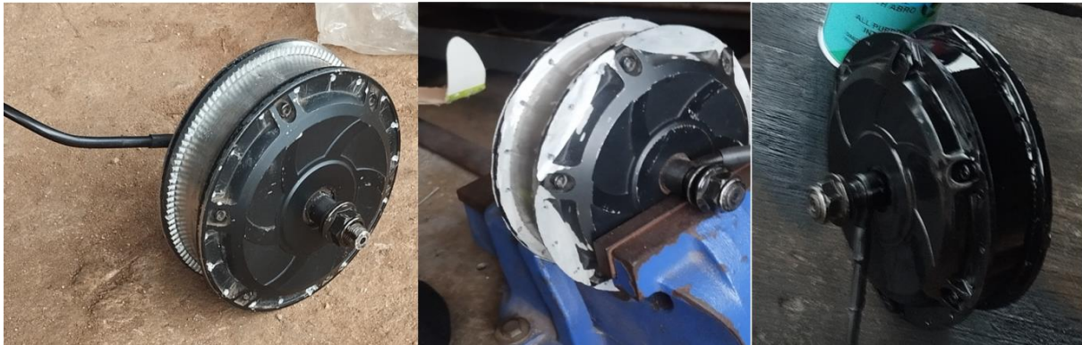
Figure 4: Drilling, grinding, and painting operation of hub motor.
