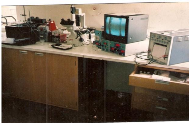
Figure 3. Pressurized vessel set up. The mesenteric artery is viewed with an inverted microscope (on the left), connected via a video camera, to a monitor which records the luminal diameter of the vessel digitally (displayed below the screen). Constriction of the vessel results in decreased diameter which can be measured.
