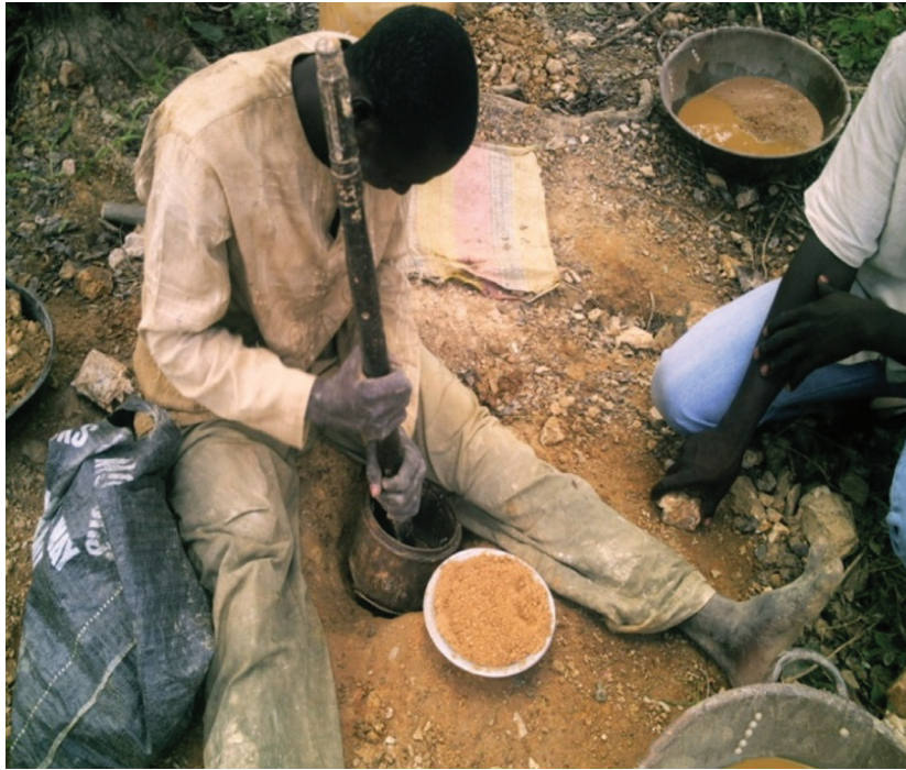
Figure1. Hand milling of ore in a mortar that could be used for milling food.
