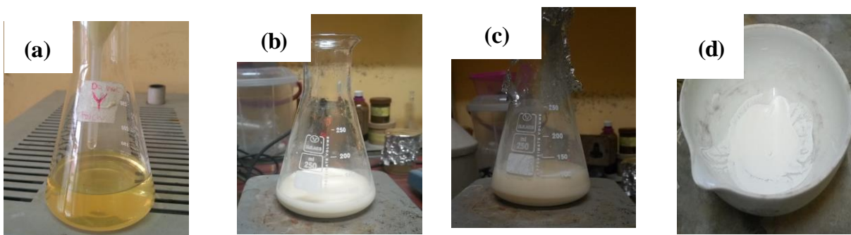
Figure 1: (a) Lime peel extract only, (b) lime peel extract and bulk titanium dioxide solution, (c) lime peel extract and titanium dioxide solution after 7 hrs of stirring, (d) Titanium dioxide nanoparticles.
