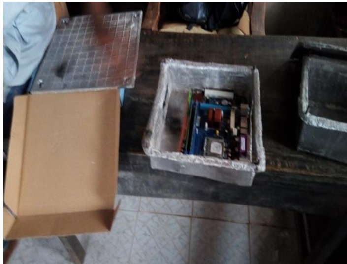
Figure 3 – Motherboard being placed in Aluminium casing.
