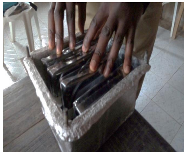
Figure 2 – Insertion and placement of hard disk array in the Aluminium casing.
