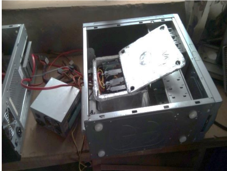
Figure 5 – Hard Disk Drives in Aluminium casing (with slanted lid) showing connecting cables to the motherboard in the next AT
