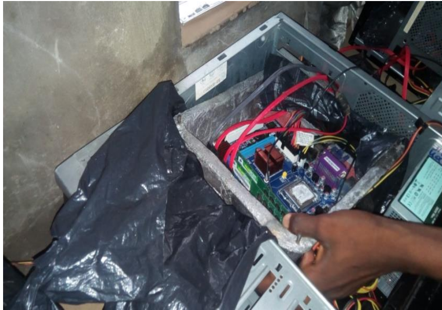
Figure 10 – Motherboard placed in aluminium casing being placed into the plastic plane and the ATX form factor casing.
