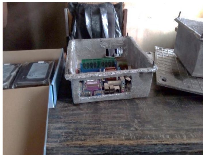
Figure 4 – Motherboard in Aluminium casing showing opening on casing side. The opening provides pathway and passage for connecting signal cable.
