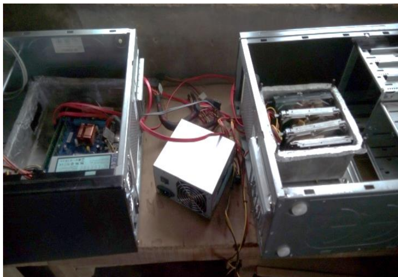
Figure 6 – Two ATX form factor desktop casing with motherboard (left) and hard disk drive (right) and power pack (middle).
