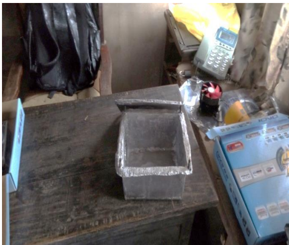
Figure 1 – Aluminium casing used to host computing system components for enhanced heat transfer.
