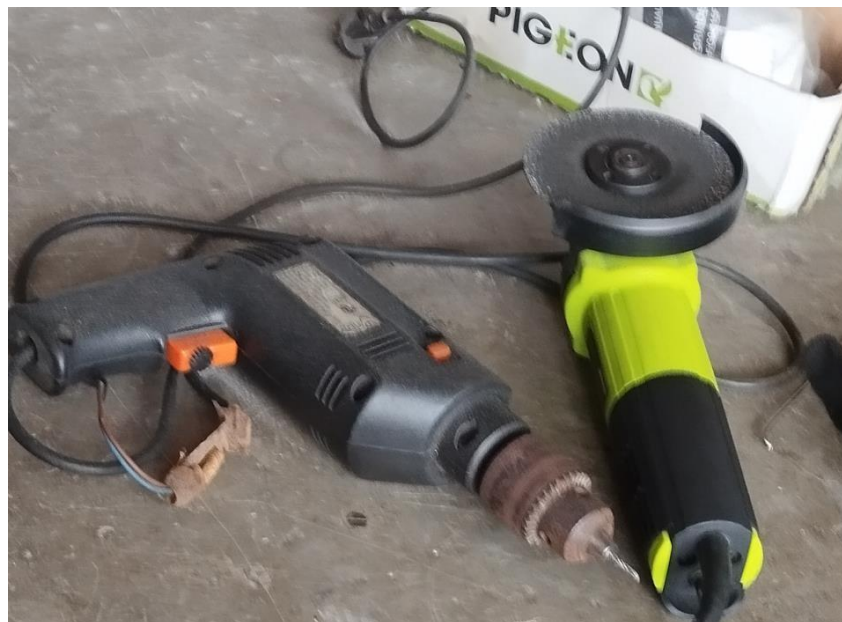
Figure 3: hand drilling and grinding machine.
